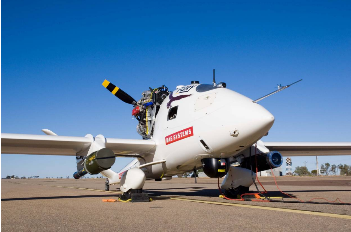
Fury on the Flight Line at Woomera (note the Camera Pod on the port pylon).
